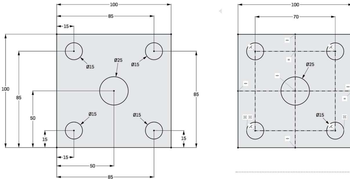
Adding design intent using geometric constraints
