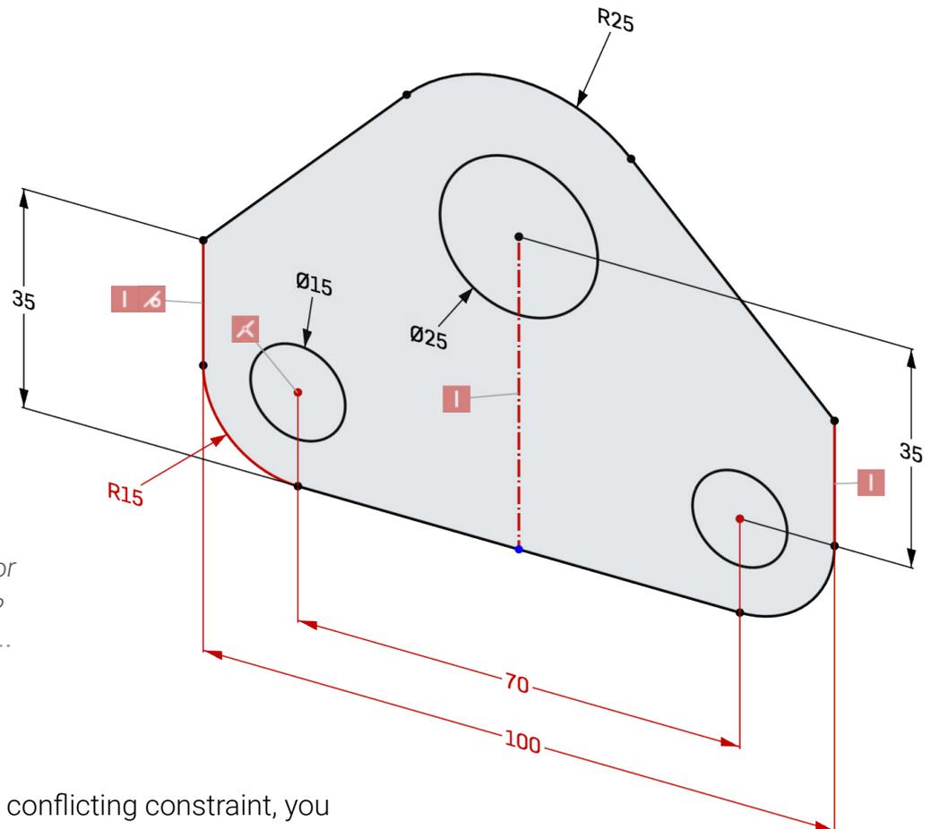
Which of these dimensions or constraints are not required?
